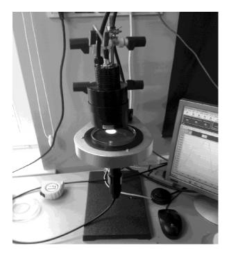
Fig. 1. A tec5 AgroSpec spectrometer applied in tests
